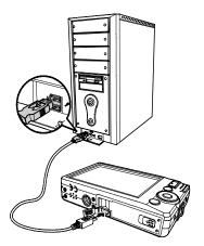
The USB Mode menu appears on the screen. Select Computer by using the ▲ or ▼ key and press the SET button.
